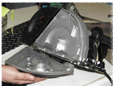
Unique cover design collects over 90% of the chips and sparks
